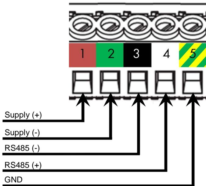
Figure 7: Connections for RAVEN-EYE®
