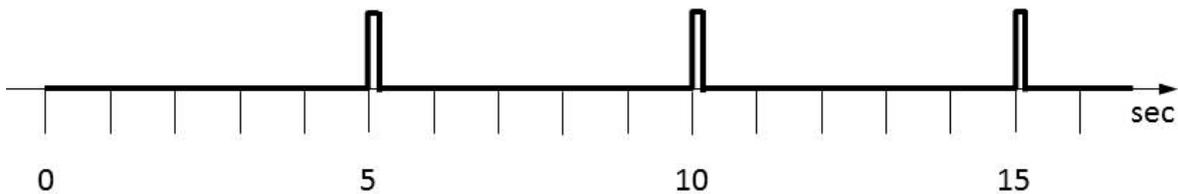
Figure 20: Contact totalizer output for 1l/s and a pulse each 5l.
