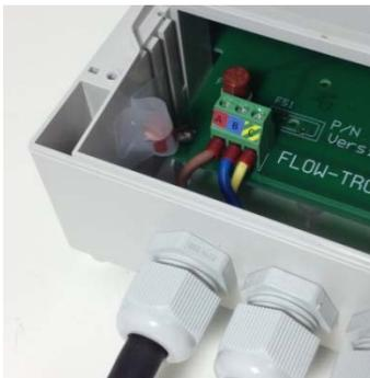
Figure 4: AC power wiring
